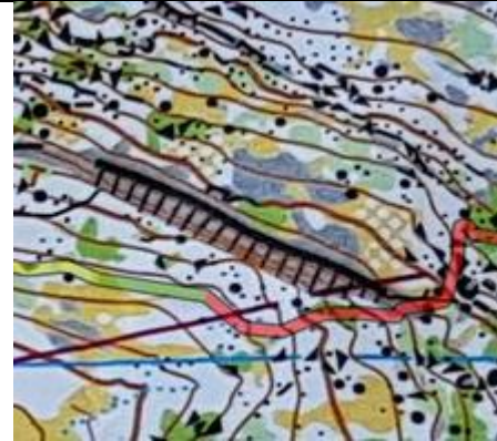
Saddleback map with steeply sloping granite bare rock with a convex slope at the top. This means it is fairly easy to start going down the cliff face and to find yourself in a very dangerous situation. Saddleback does have quite a few boulders shown using the 206 Gigantic boulder or rock pillar symbol. Using 206 for this cliff could be quite dangerous.
